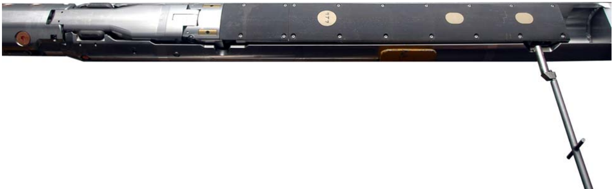
FIGURE 9-3 The Atlas Densilog, which uses an Am-Be source for wireline density measurements. The rod extending downward is a source handling device used for source insertion and removal. The light-colored circles are windows for the source and detectors. SOURCE: Photo courtesy of Baker Hughes Incorporated.
