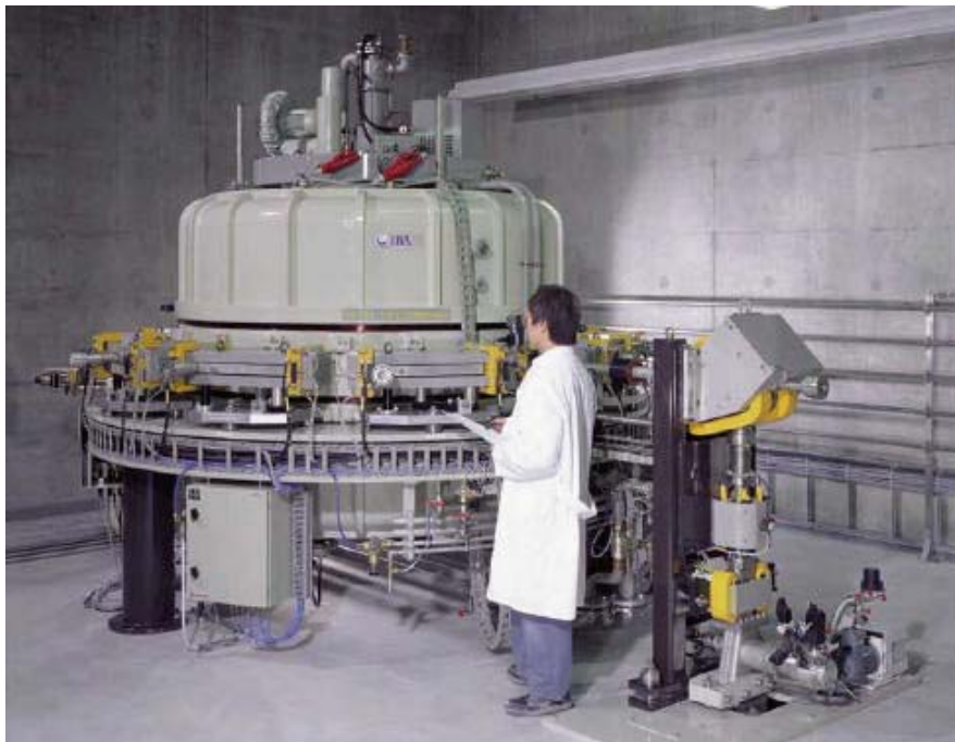
FIGURE 4-7 Picture of a 200 kilowatt Rhodotron used to irradiate U.S. mail at a facility in New Jersey. SOURCE: Image courtesy of IBA-RDI.
