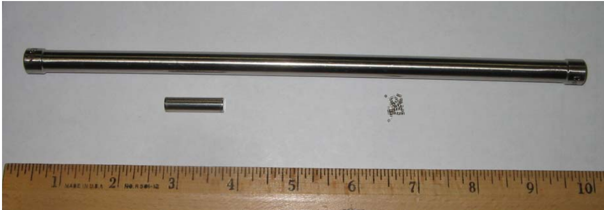
FIGURE 2-1 A photograph of a typical cobalt-59 pencil and slug, which is irradiated to make industrial cobalt-60 sources. Also, a pile of cobalt-59 pellets, which can be irradiated in a high-flux reactor to make cobalt-60 teletherapy, and, and industrial radiography sources. The ruler uses English units (1 inch = 2.54 cm).
