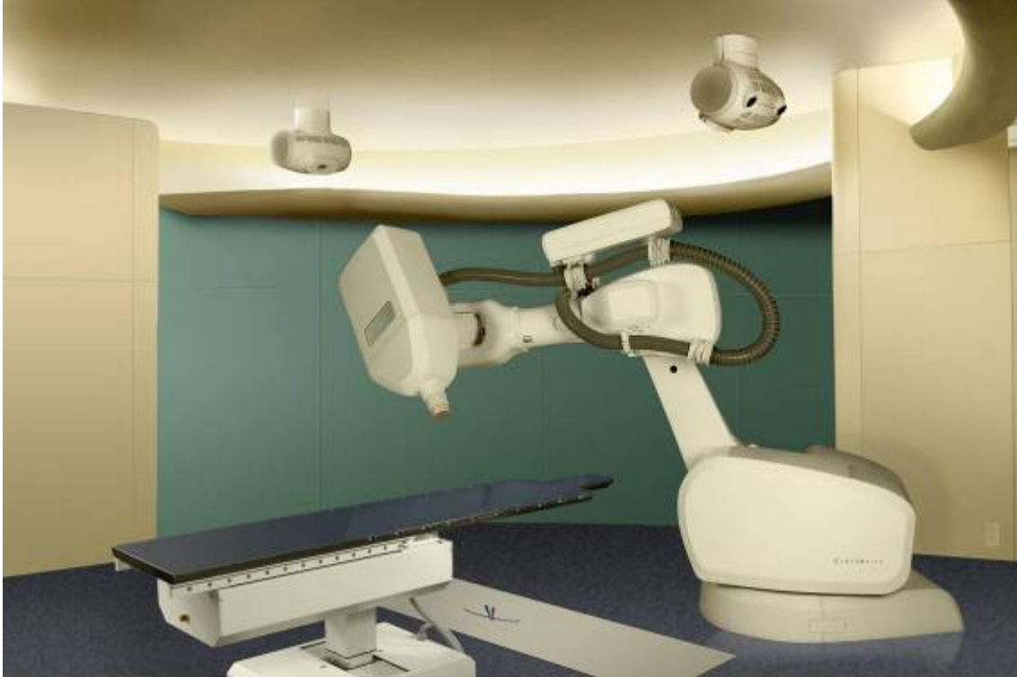
FIGURE 7-9 CyberKnife® installation consisting of miniature linac mounted on a robotic arm, treatment couch, and imaging device: ceiling-mounted x-ray tubes and floor-mounted image intensifiers. SOURCE: Courtesy of Accuray, Sunnyvale, CA.
