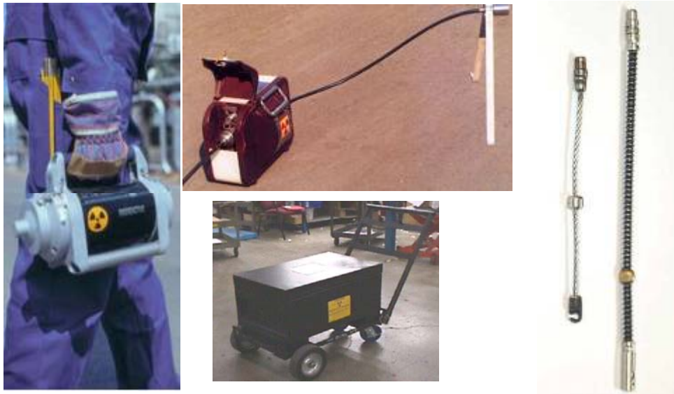
FIGURE 8-3 Radiography Cameras. Note that the hand held device is an iridium-192 radiography camera, as is the sealed source mounted on the end of the cable shown to the right. The device on wheels is a cobalt-60 radiography camera.
