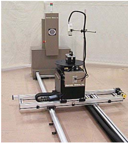
FIGURE 5-7 Typical gamma calibrator configuration for survey instrument calibration. SOURCE: Hopewell Designs (2007).
