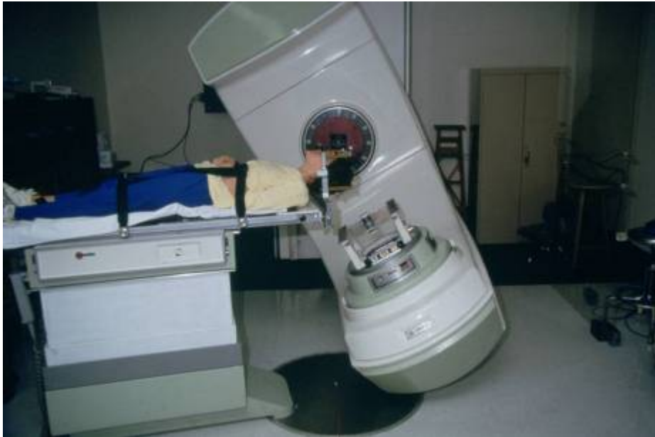
Figure 7-7: Patient receiving linac-based dynamic stereotactic radiosurgery on a Clinac 18, a linac manufactured in the 1970s by Varian Medical Systems. More recent medical linacs developed specifically for stereotactic radiosurgery incorporate image-guidance and beam-shaping technologies.
