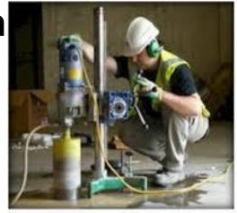
Concrete coring to obtain samples for evaluating effects of aging and environmental stressors
