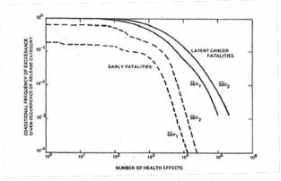
Figure 2 Conditional Risk Curves for Early and Latent Fatalities for Single  $(S6V_1)$  and Double  $(S6V_2)$ Core Melts with Large Isolation Failure
