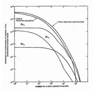
Figure 4 Risk Curve (CCDF) for Latent Cancer Fatalities for Two Unit Reactor Station
