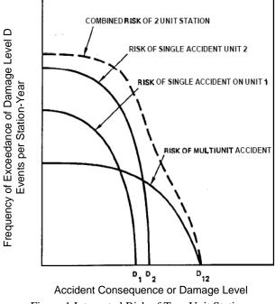
Figure 1 Integrated Risk of Two Unit Station
