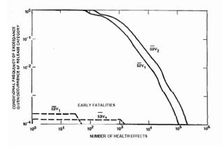
Figure 3 Conditional Risk Curves for Early and Latent Fatalities for Single  $(S2V_1)$  and Double  $(S2V_2)$ Core Melts with Small Isolation Failure
