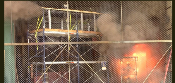
Brown smoke visible from test with copper electrodes
