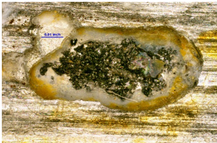
Pit picture with 100x magnification; pit reached absorber material
