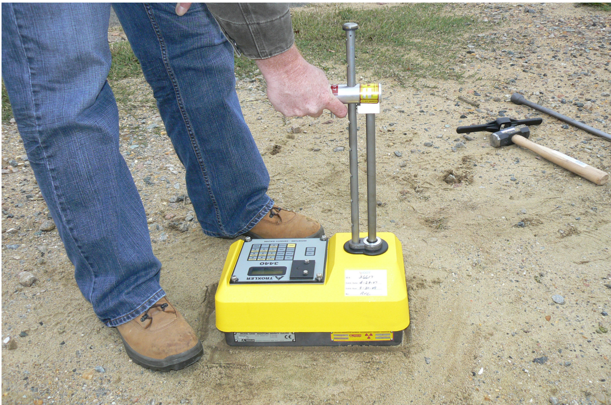
A moisture density gauge indicates whether a foundation is suitable for constructing a building or roadway. Photo courtesy of the American Portable Nuclear Gauge Association.
