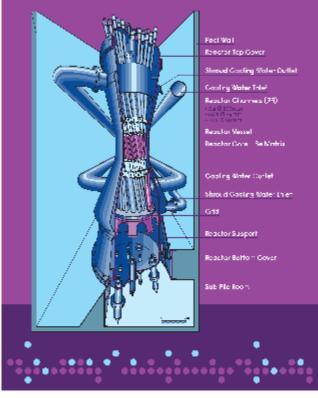
Top Left: TREAT Reactor at INL (Copyright © INL). Bottom Left: LVR-15 Reactor / CVR (Czech Republic). Right: BR2 Reactor Diagram / SCK-CEN (Belgium)
