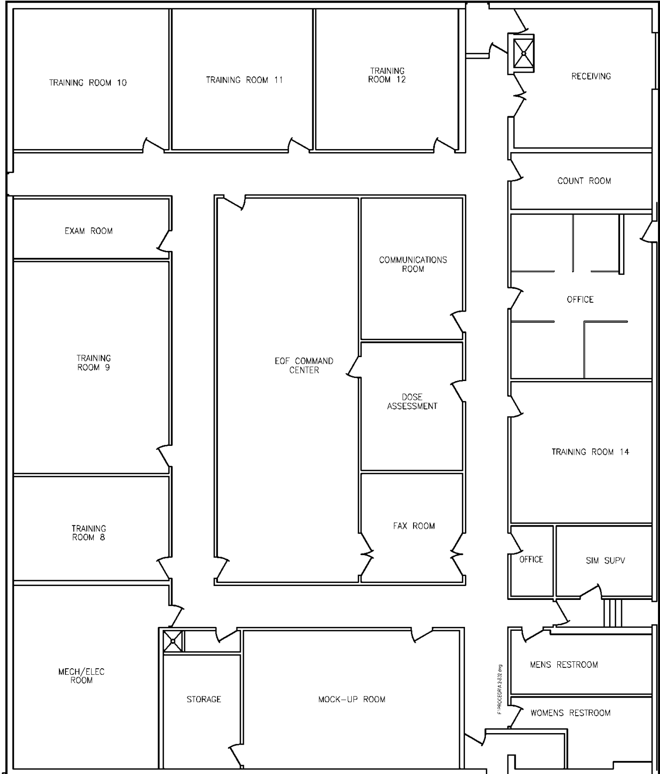
Figure 13.5 PLAN VIEW OF THE EMERGENCY OPERATIONS FACILITY
