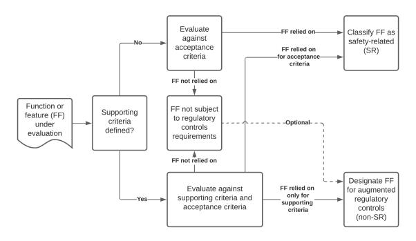
Figure 4-1: Classification of functions and features
