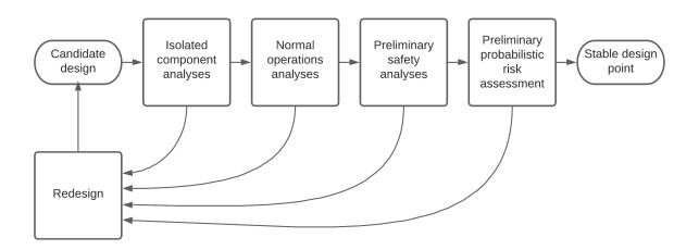
Figure 2-1: Iterative design process
