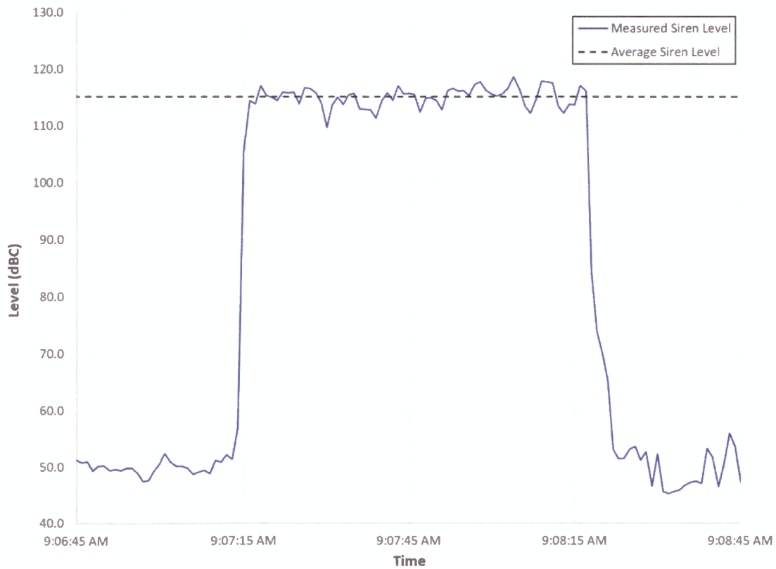
Figure 34. Time history of the received sound from siren 522 as measured from the bucket truck
