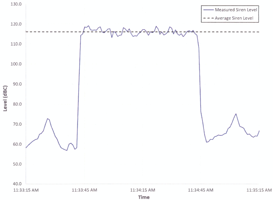
Figure 54. Time history of the received sound from siren 3Z5 as measured from the bucket truck
