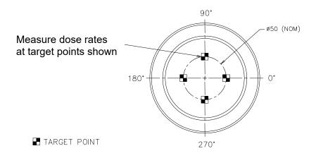
Measure dose rates at eight target points (0, 45, 90, 135, 180, 225, 270 and 315 degrees) on each plane, at center of each inlet and outlet and at a point in between each inlet and outlet.
