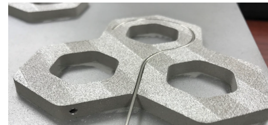
316L sheathed sensor in AM 316L build
