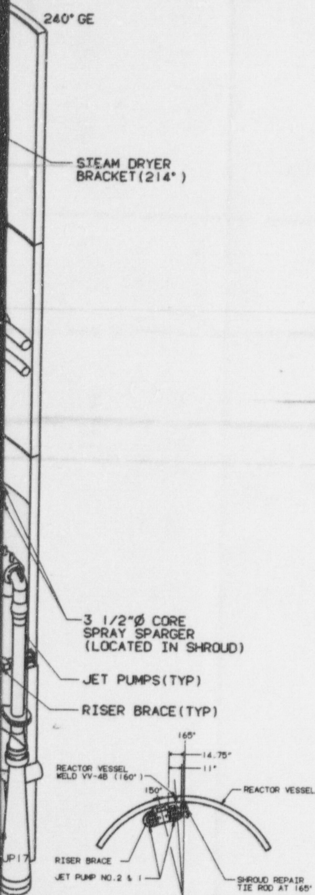
PART PLAN SHROUD REPAIR TIE ROD (165") AND JET PUMP RISER BRACE
