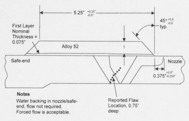
First layer thickness can be less than 0.075-inch if surface passes surface PT examination.
