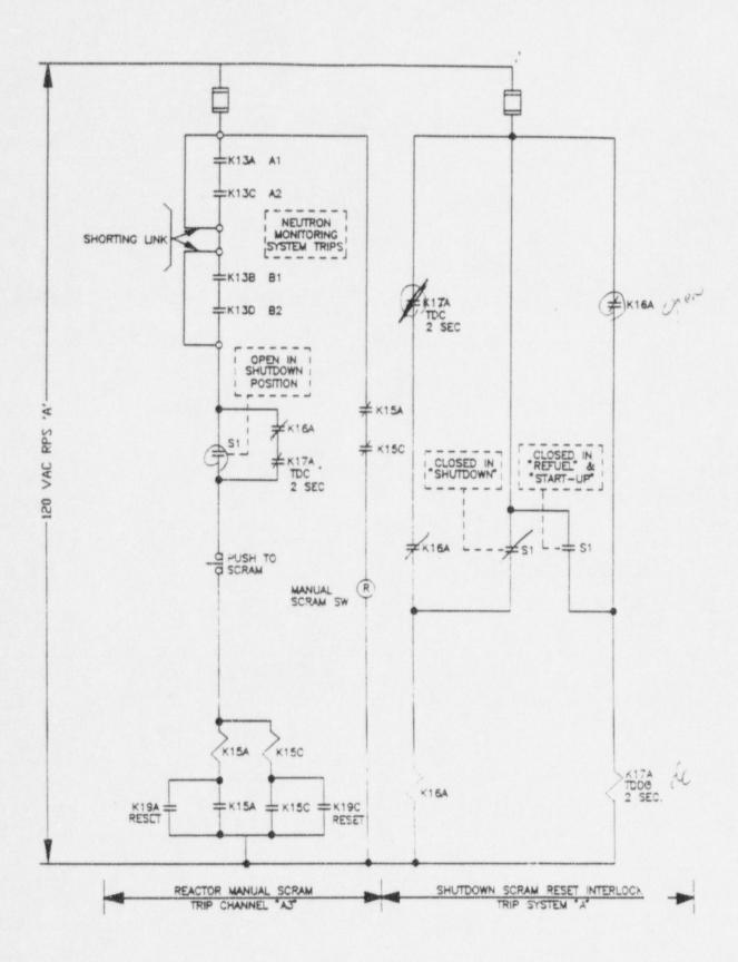
Figure 03-21 - Shutdown Scram Reset Interlock
