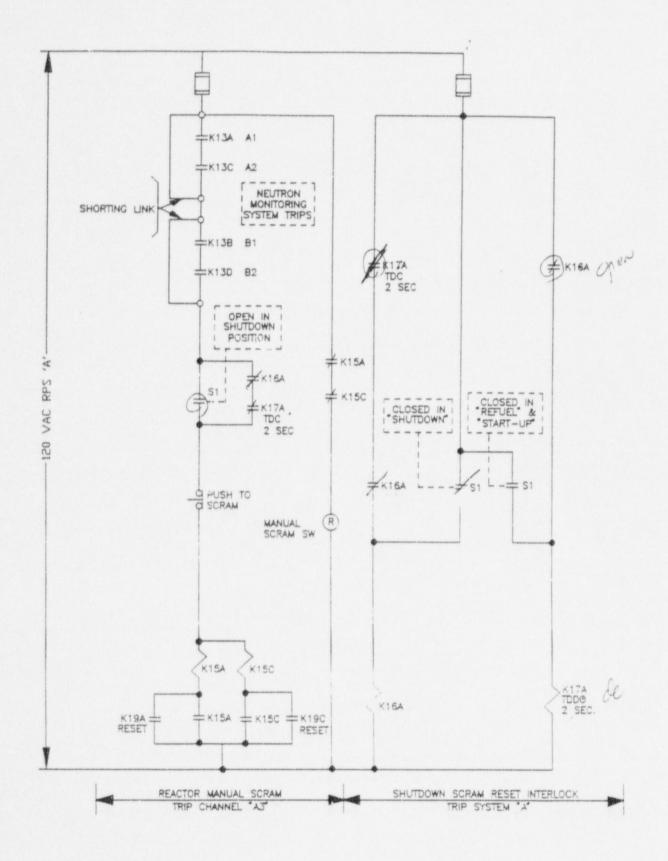
Figure 03-21 - Shutdown Scram Reset Interlock
