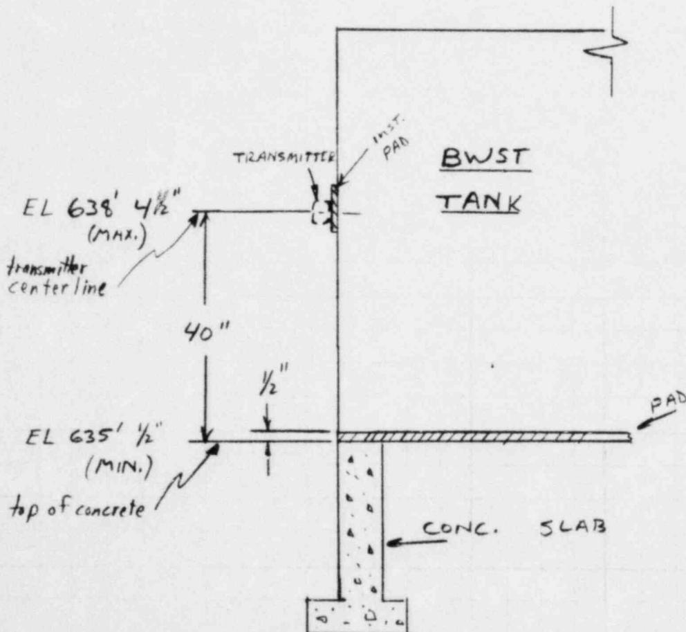
USING INFO. ABOVE THE SPAN OF THE TRANSMITTER IS CALCULATED BY SUBTRACTING THE HEIGHT OF THE TRANSMITTER FROM THE HEIGHT OF THE TANK (384"). THIS TURNS OUT TO BE  $384" - 40" = 344"$ . THIS SHALL BE USED FOR THE TRANSMITTER CALIBRATED RANGE.
