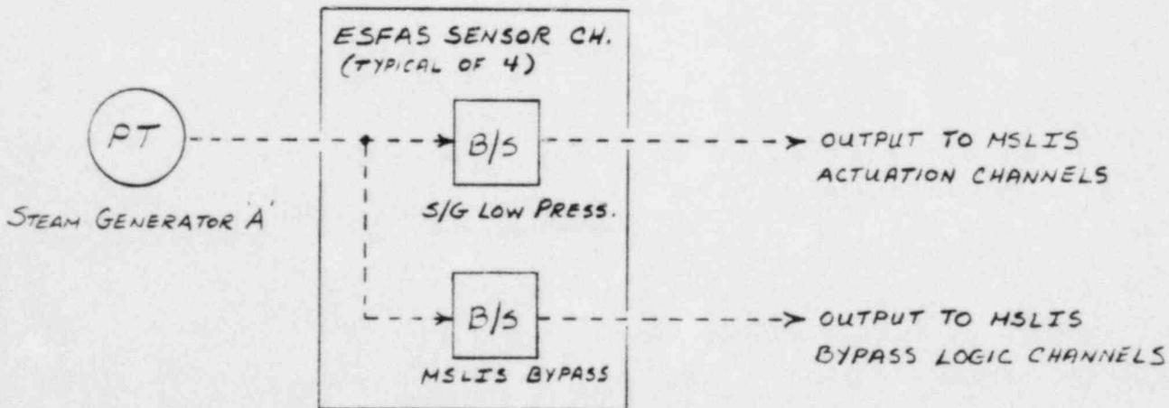
A block diagram of a typical steam generator 'B' loop would be identical to the above diagram.
