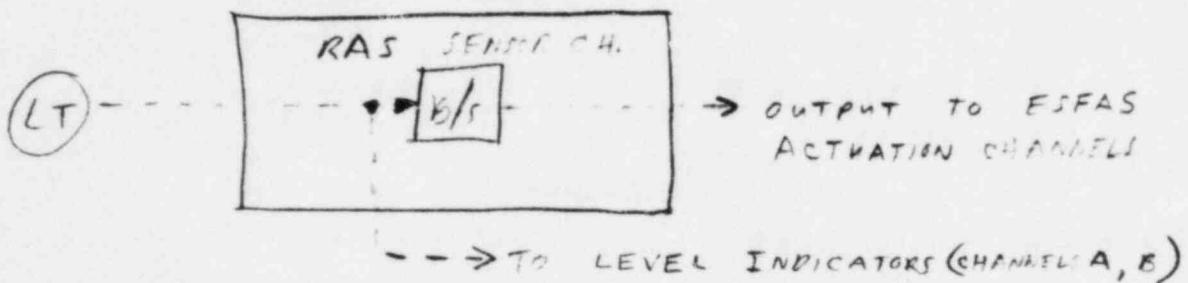
The calculation which follows will consider the combined effects of transmitter and bistable module tolerances on the determination of the low level setpoint and allowable values.
