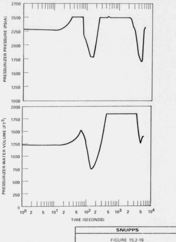
PRESSURIZER PRESSURE AND WATER VOLUME TRANSIENTS FOR MAIN FEEDWATER LINE RUPTURE WITH OFFSITE POWER AVAILABLE
