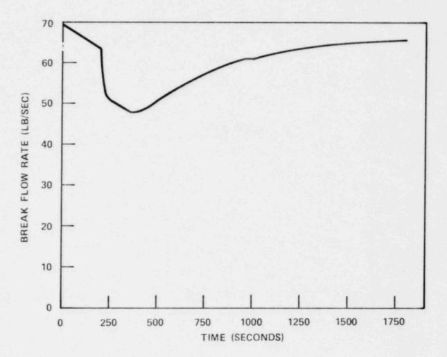
Figure 15.6-31. Faulted Steam Generator Break Flow Rate Transient for Steam Generator Tube Rupture Event
