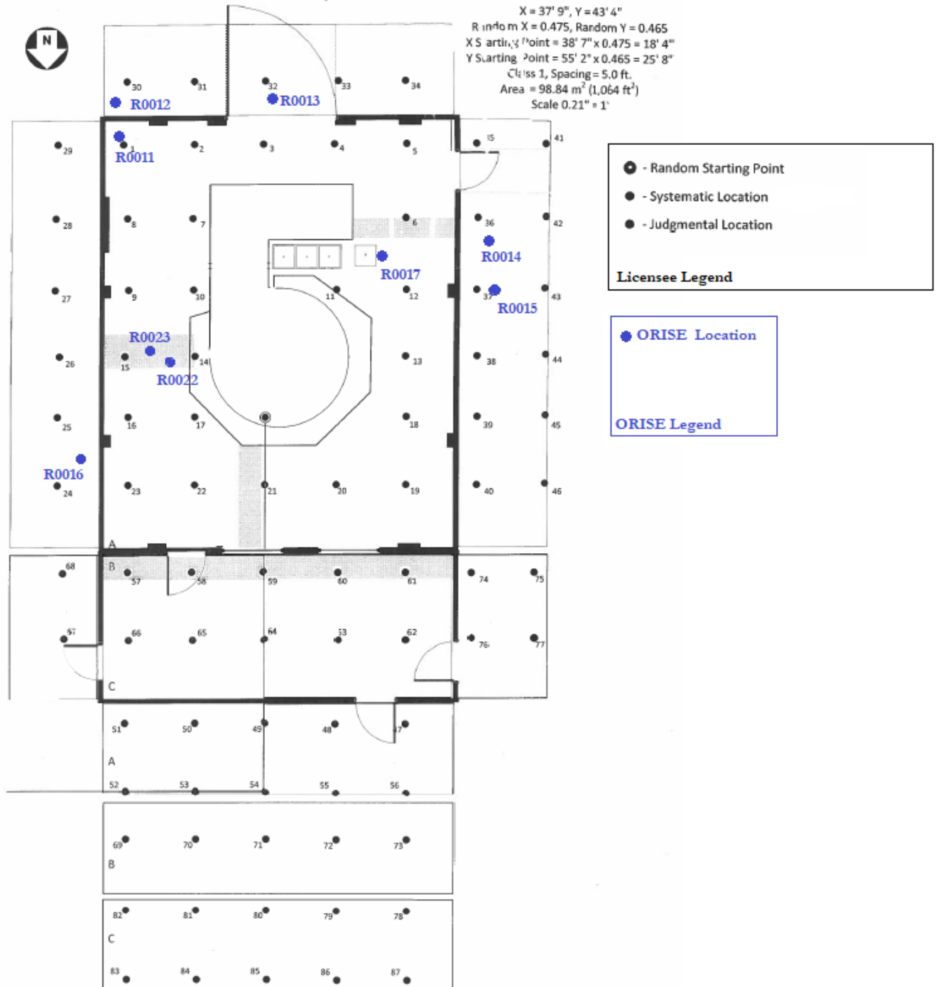
Figure A.5. SU 5 Mark F Reactor Room (floors and lower walls) Survey Locations
