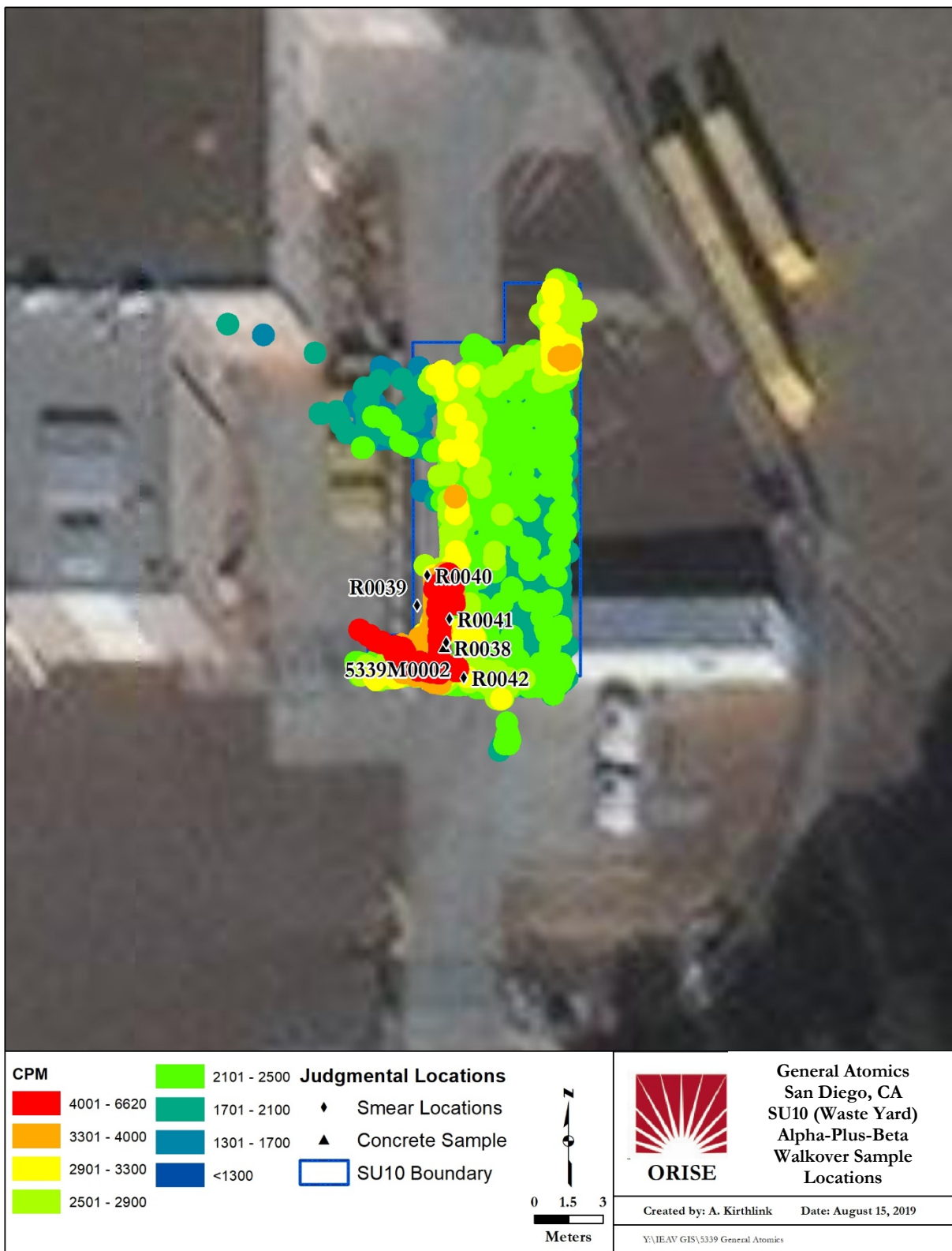
Figure A.10. SU 10 TRIGA Waste Yard Alpha-Plus-Beta Walkover Map with Survey Locations
