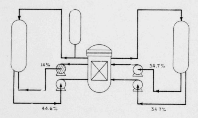
. FIGURE 1 Reactor Coolant System Flow for 3-pumps operating (percent of total system flow).
