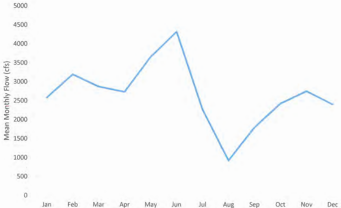
FIGURE 7: Mean Monthly Flow (cfs) by Month from 1948-2008 at USGS 08162500 Colorado River near Bay City, TX
