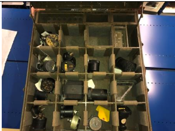
B-10. Case with discrete sources of Ra-226 in the Main Campus Archive Area
