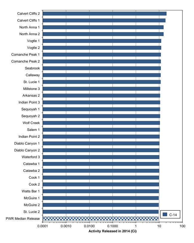
Figure 3.10 PWR Gaseous Releases — Carbon-14
