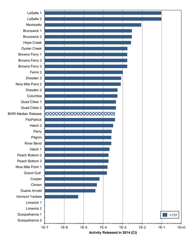
Figure 3.2 BWR Gaseous Releases — Iodine
