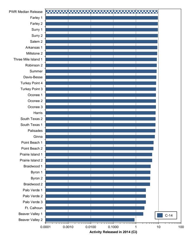
Figure 3.10. PWR Gaseous Releases — Carbon-14 (continued)
