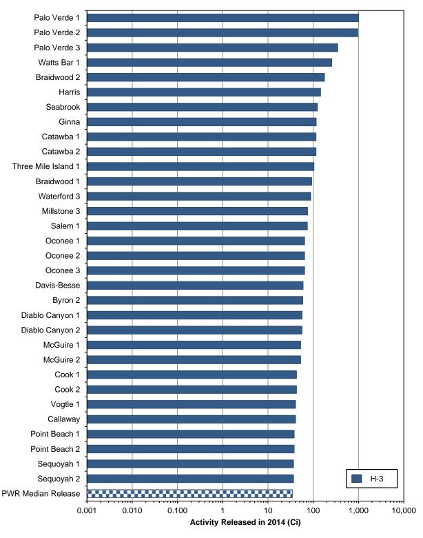
Figure 3.9 PWR Gaseous Releases — Tritium
