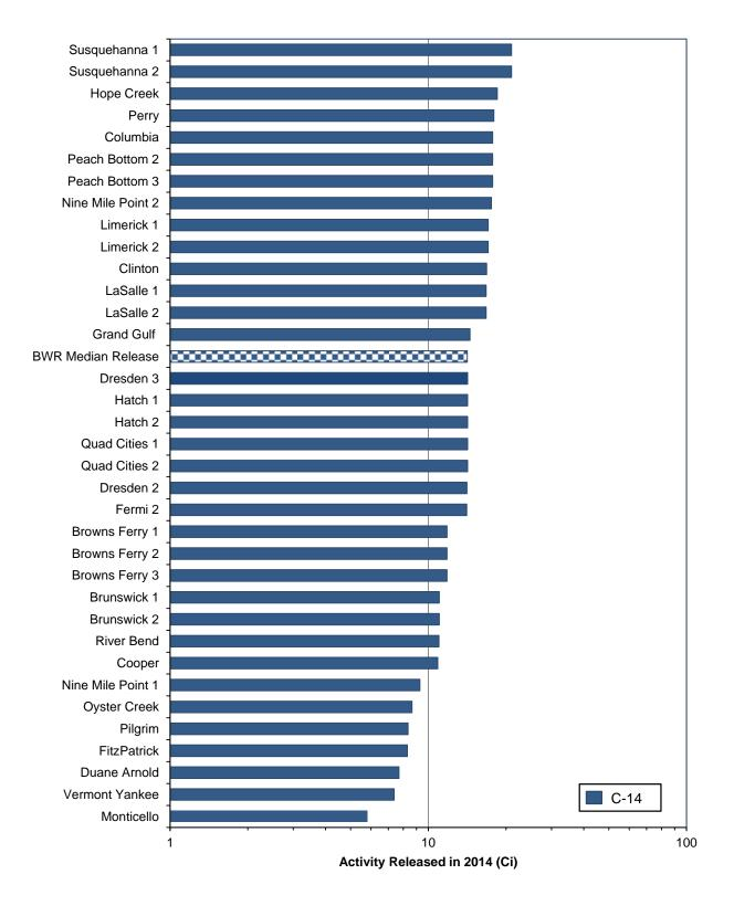
Figure 3.5 BWR Gaseous Releases — Carbon-14
