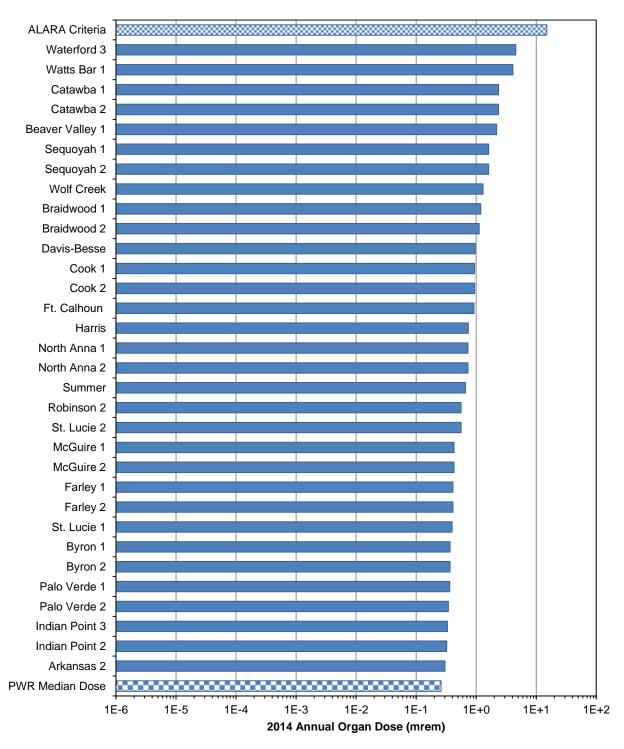
Figure 3.18 PWR Gaseous Effluents — Maximum Annual Organ Dose
