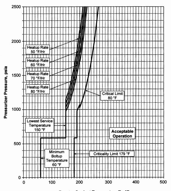
$\label{eq:continuous} \textbf{Reactor Coolant Temperature T}_{c},\,^{\circ}\textbf{F}$  (Curves do not include margins for instrument uncertainties)
