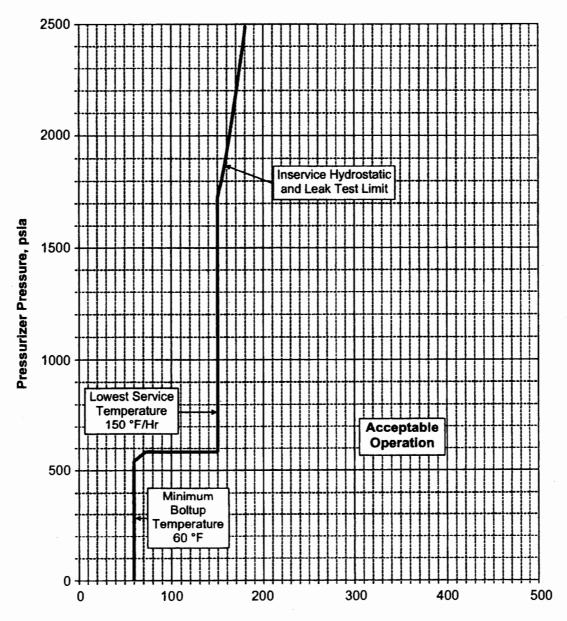
$\label{eq:Reactor Coolant Temperature T} \textbf{C}, \ ^{\circ}\textbf{F}$  (Curves do not include margins for instrument uncertainties)
