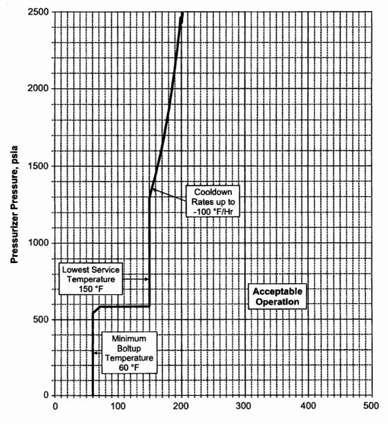
$\label{eq:Reactor Coolant Temperature T_c, °F} \\ \text{(Curves do not include margins for instrument uncertainties)}$
