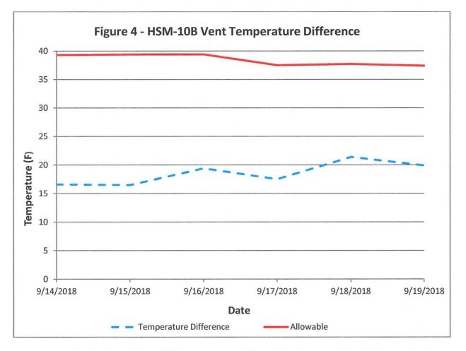
The system reached thermal equilibrium on or before September 19, 2018. At that time the temperature difference across the inlet and outlet vents was 19.9°F. This is below the acceptance criteria of 37.4 °F. MNGP has determined the system is functioning as designed.
