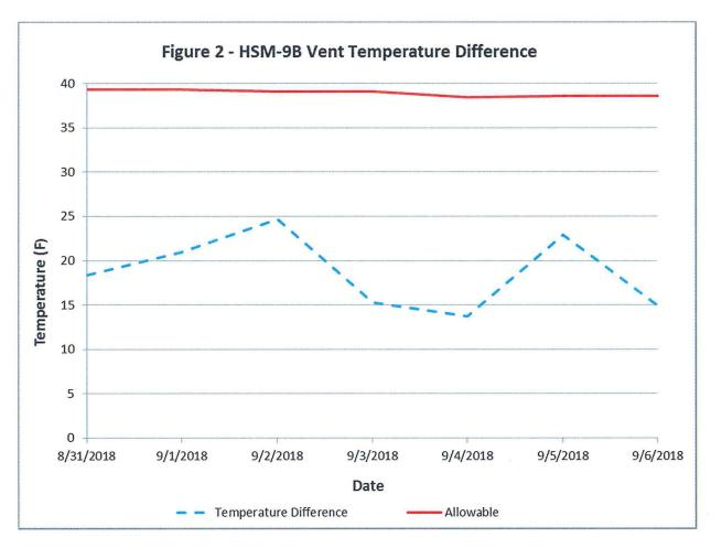
The system reached thermal equilibrium on or before September 4, 2018 with additional data collected through September 6, 2018 for trending. On September 6, the temperature difference across the inlet and outlet vents was 14.9°F. This is below the acceptance criteria of 38.6°F. MNGP has determined the system is functioning as designed.
