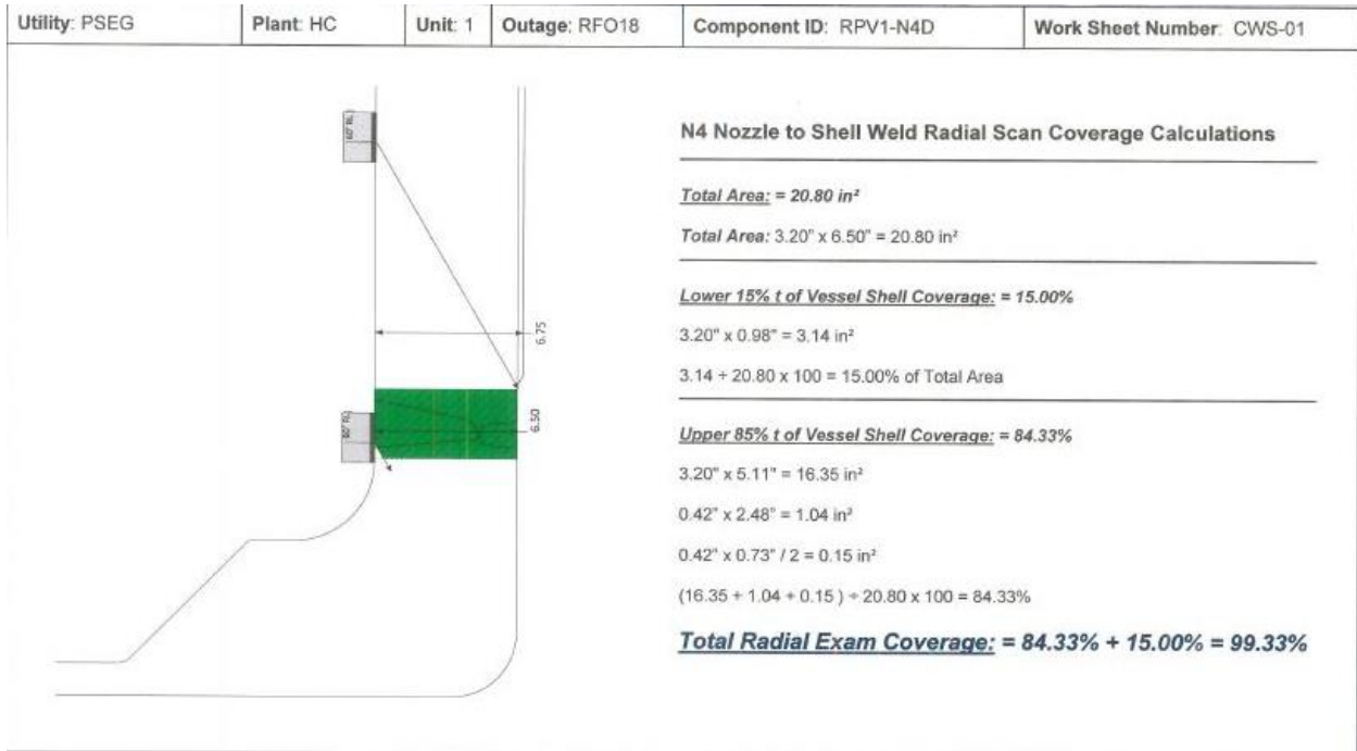
Figure 1.9-2 Weld RPV1-N4D (Radial Scans) Coverage Calculations from Shell Side
