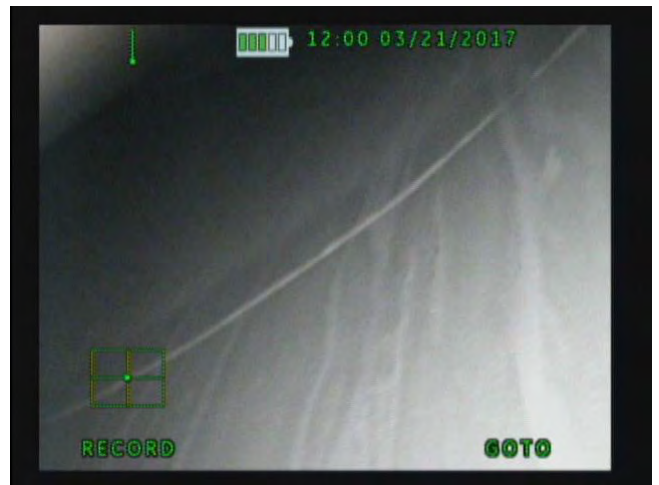
4. Vault Liner Weld
