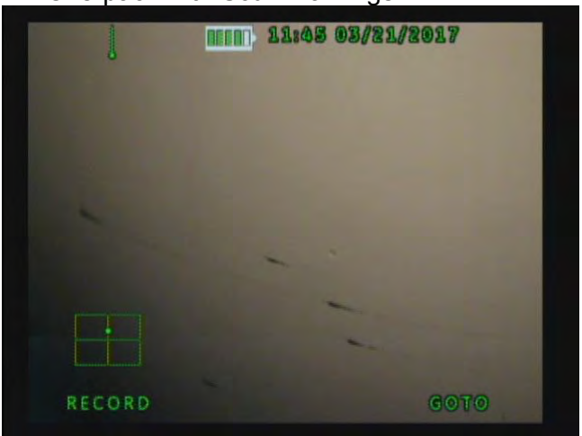
17. Overpack with Scuff Markings
