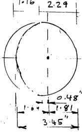
CG of corroded section
