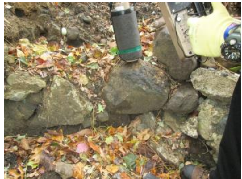
Figure A-16. Rock with Elevated Radiation Levels (due to NORM)
