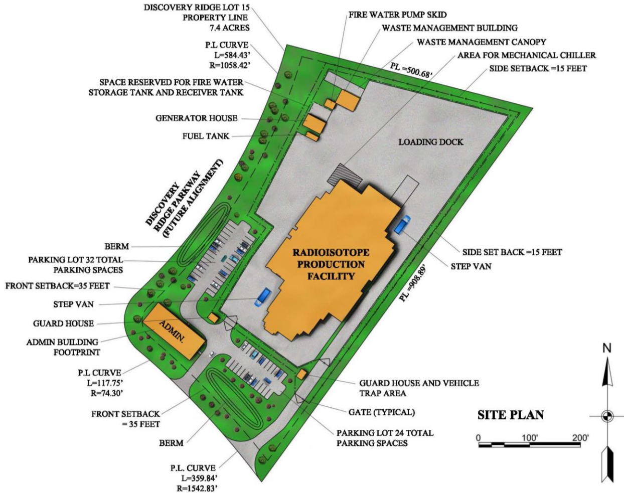
Figure 2-5. Radioisotope Production Facility Site Layout
