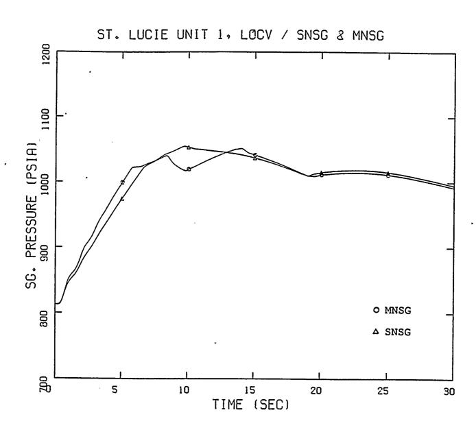
FIGURE 3. ST. LUCIE 1, STEAM GENERATOR PRESSURE
