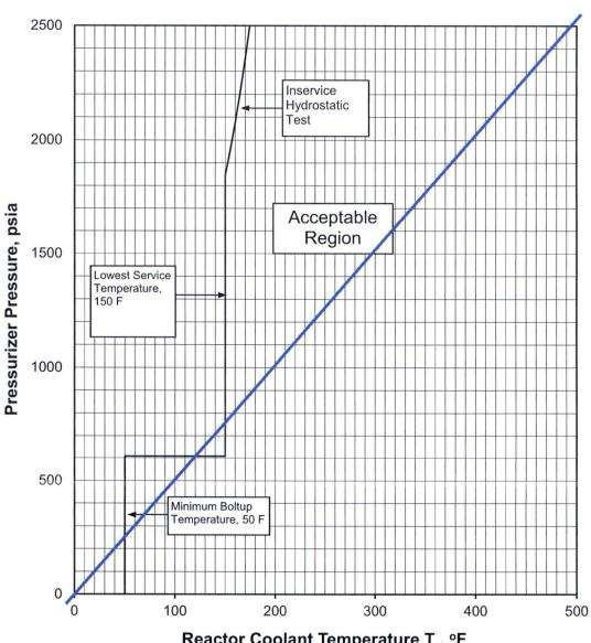
**INSERVICE HYDROSTATIC TEST CURVE**:- 3254 REACTOR COOLANT SYSTEM PRESSURE/TEMPERATURE LIMITS
