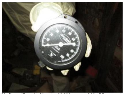
A-10. Gauge Found with up to 30,000 cpm and 16 μR/h on contact
