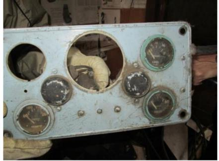
A-11. Gauges Found with Measurable Exposure Rates up to 100 μR/h on contact
