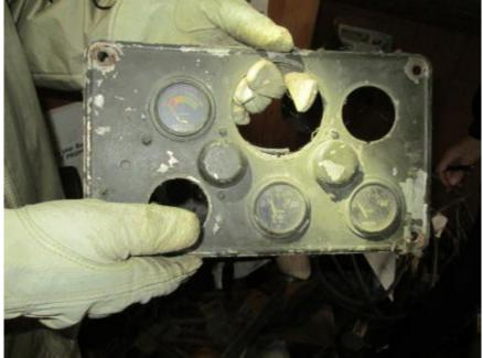
A-12. Gauges Found with Measurable Exposure Rates up to 100 μR/h on contact
