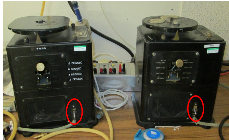
A-6. Turntables T539 (left), T549 (right). Toggle switches with elevated levels of radiation circled in red.
