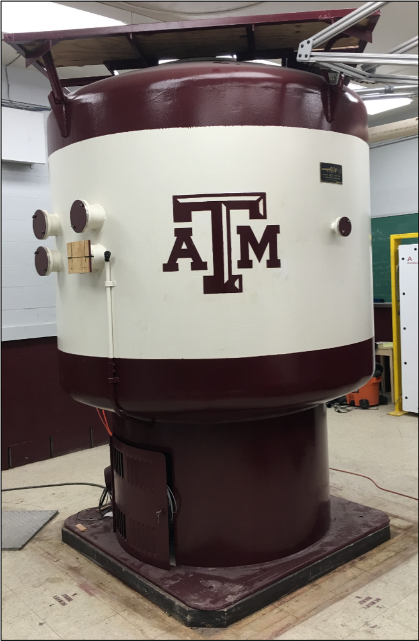
Figure 2a – AGN-201M Reactor without block shielding, as currently located in Zachry Engineering Center
