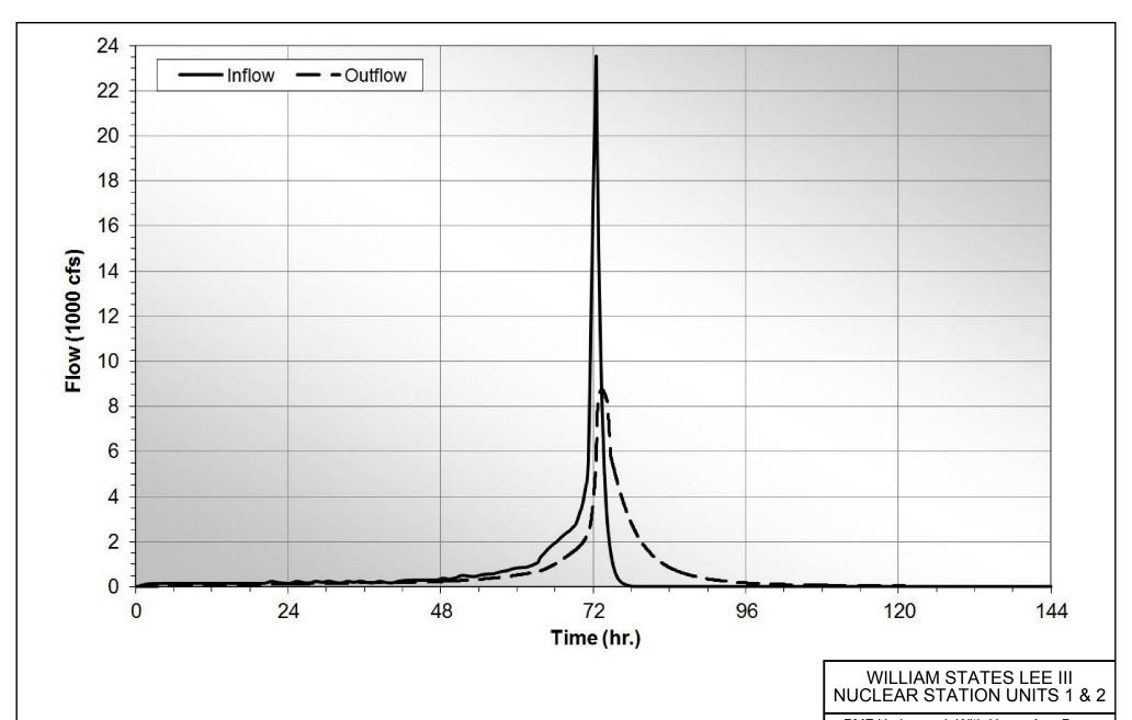
PMF Hydrograph With Upper Arm Dam Failure, Make-Up Pond B
