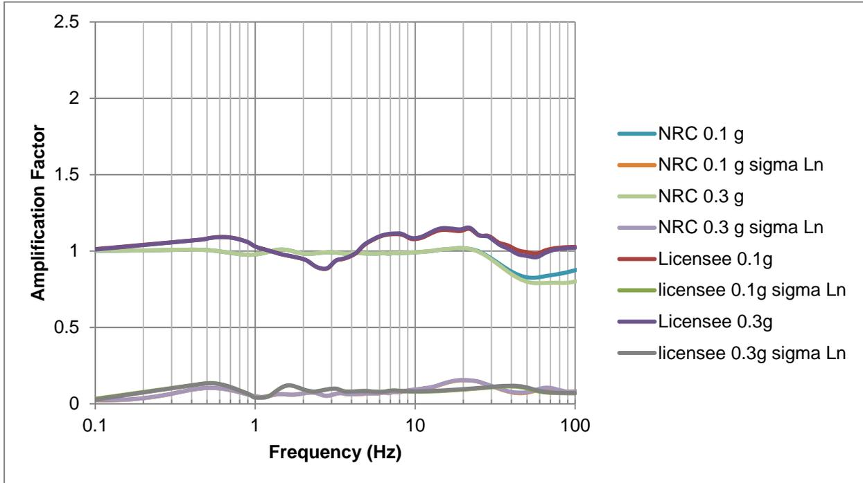
Figure 3.3-3 Plot Comparing the Staff's and the Licensee's Mean Control Point Hazard Curves at a Variety of Frequencies for the Oconee site
