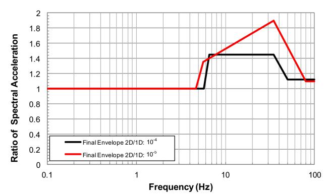
Figure 3.7.1-215 FWSC 2D/1D Response Spectral Ratios for Fill Concrete [EF3 COL 2.0-27-A, EF3 SUP 3.7-1]
