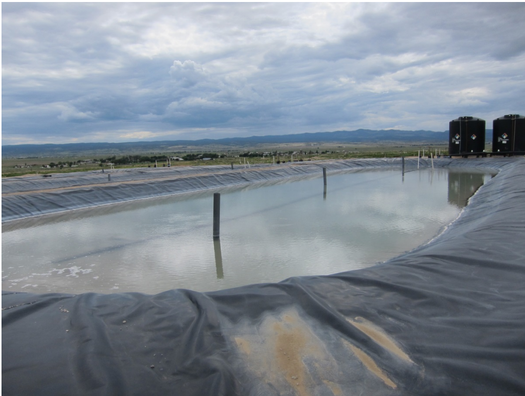
Figure 2: One of three zeolite pilot test system treatment cells
