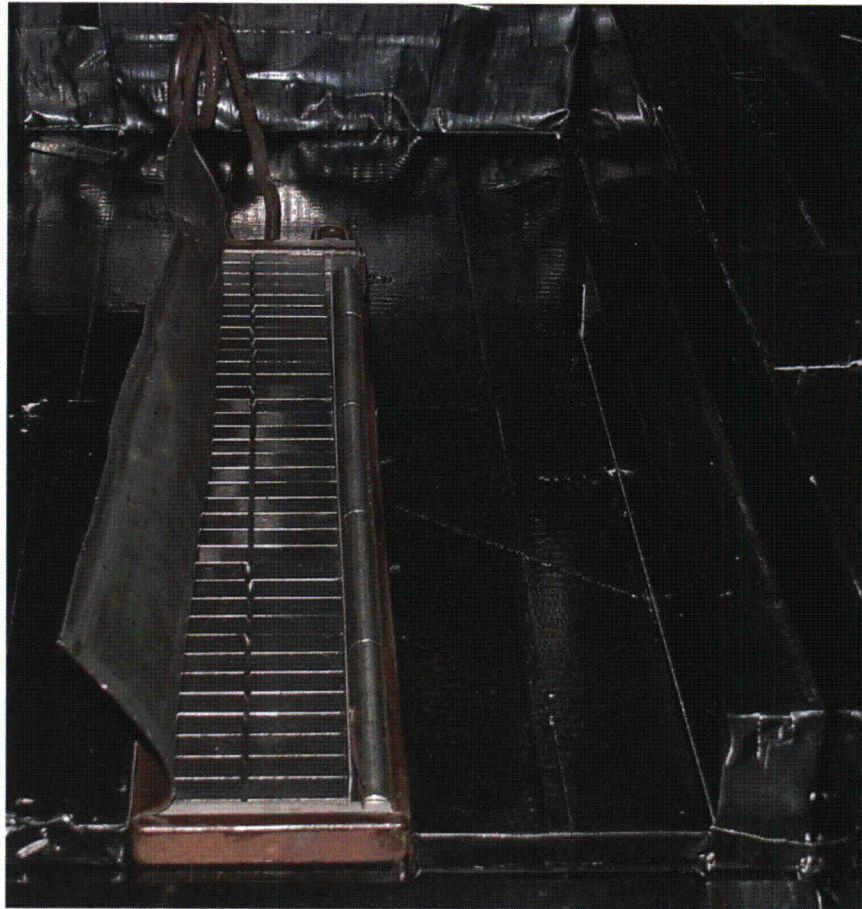
Figure 2-3 Photograph of the Inside of the 177 Degree Perry Capsule Showing the Dosimetry Location During the Irradiation
