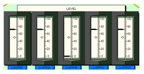
The Plant is at 100% power. RPS Channel B for 'A' Steam Generator Low Level is BYPASSED due to a failure of LI-0751B.
