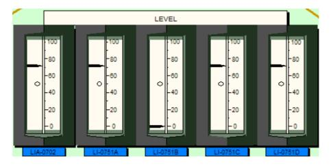
The Plant is at 100% power. RPS Channel B for 'A' Steam Generator Low Level is BYPASSED due to a failure of LI-0751B.
