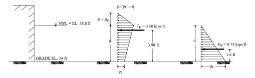
$F_D$  = Resultant hydrodynamic force (in kips per linear foot) equivalent to the hydrodynamic wave pressure ( $p_1$  and  $p_2$ ) acting on the structure
