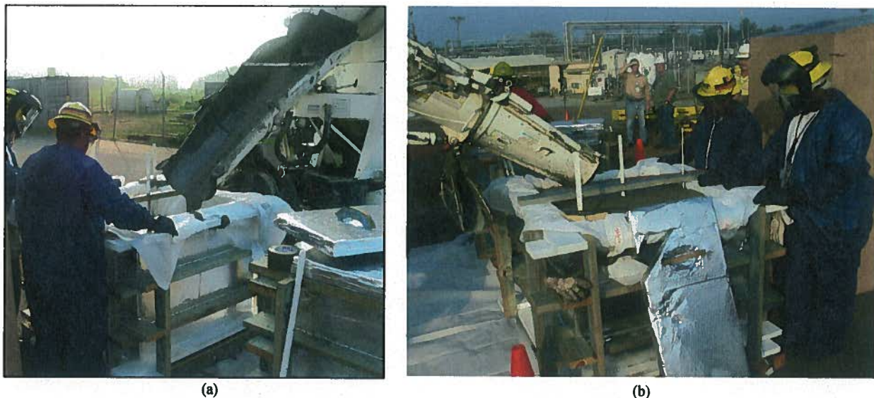
Figure 2-4. (a) Bulk tank fill grout placed into the semi adiabatic form and (b) Near full form.
