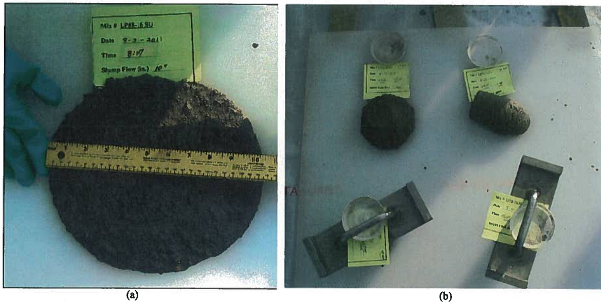
Figure 3-1. Spread under static conditions, (a) initial, (b) Top left 15 minutes, Top right 30 minutes.
