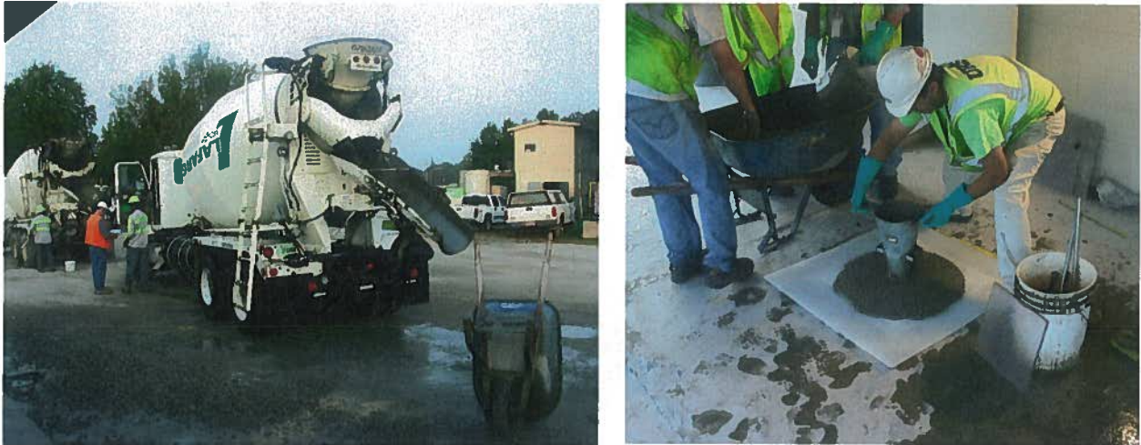
Figure 2-2. Admixture dose adjustment at the LaFarge batch plant based on ASTM C1611 test results.
