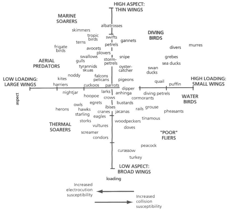
Figure 5. Estimated bird group electrocution and collision susceptibility with power lines based on principal components analysis of wing size and wing proportions.
