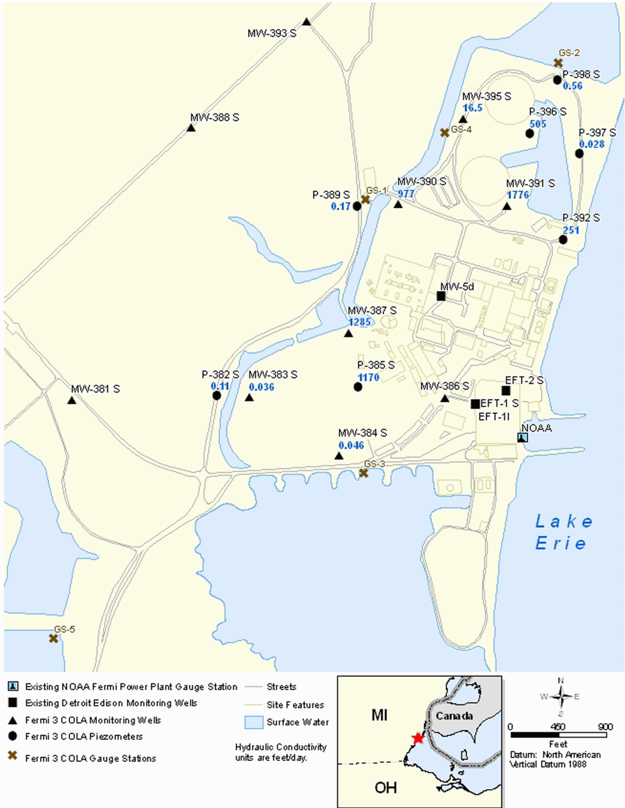
Figure 2.4-252 Fermi 3 Overburden Hydraulic Conductivity [EF3 COL 2.0-23-A]
