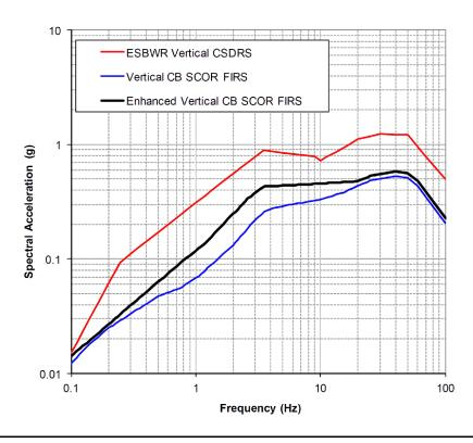
Figure 2.0-203 Horizontal and Vertical FWSC FIRS and 1.35 Times the CSDRS [5 Percent Damping] (FIRS are developed in Subsection 3.7.1)
