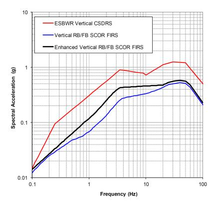
Figure 2.0-202 Horizontal and Vertical CB Enhanced SCOR FIRS and CSDRS [5 Percent Damping] (FIRS are developed in Subsection 3.7.1) [EF3 COL 2.0-1-A]
