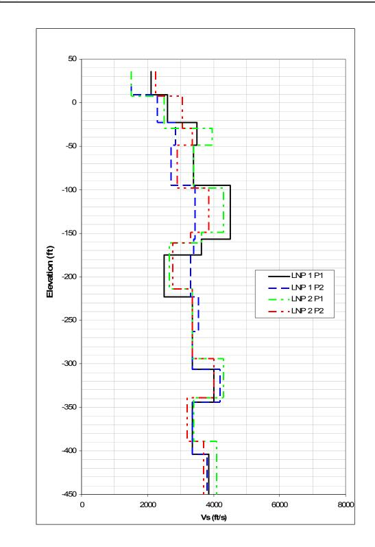
Note: Profiles LNP 1 P1 and LNP 2 P1 are based on suspension logging data Profiles LNP 1 P2 and LNP 2 P2 are based on downhole data Duke Energy Florida
