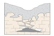
The slow, downward erosion eventually forms small surface depressions 1 inch to several feet in depth and diameter.
