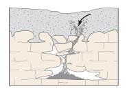
Granular sediments ravel into secondary openings in the underlying carbonate rocks.
