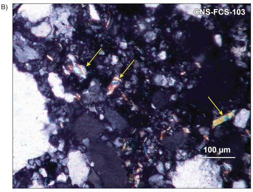
Photomicrograph thin section CNS-FC-103 (cross-polarized light). Late- to post-kinematic white mica (yellow arrows) overgrowing brittle fabric.
